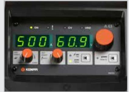
Clear and easy to use interface including LCD display, plus selection of Arc dynamics and Hot start values.
