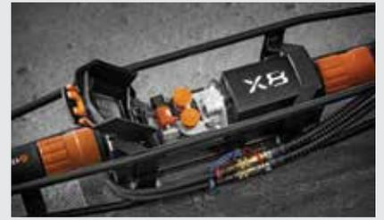
The X8 SuperSnake features a two-roll version of the X8 Wire Feeder's powerful wire feed mechanism with firm locking. The consumables are interchangeable, and color-coded to ensure that you always use the correct combination.
