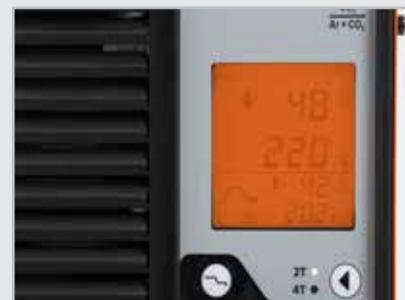
Crater fill function reduces the voltage level at the end of the weld and ensures the best arc control right to the finish. The end of the weld is nice and clean, which makes it easy to start the next weld without wasting welder's tie in grinding.
