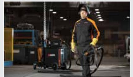
The lightweight sub-feeder is an ergonomic option for carrying heavy and large wire feeders, or welding with heavy push-pull welding guns that increase strain on the welder's wrist.
