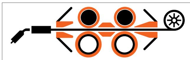
Typical wire feed mechanism
