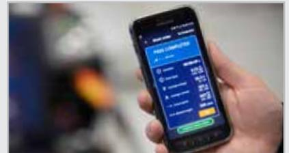
*By using the WeldEye mobile application, welders can browse their company's WPS library, receive digital work orders, report work progress, and get feedback on their welds – including heat input values.*
