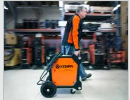
ArcValidator load bank is easy to move around and a universal solution for multi-branded fleet validation.
