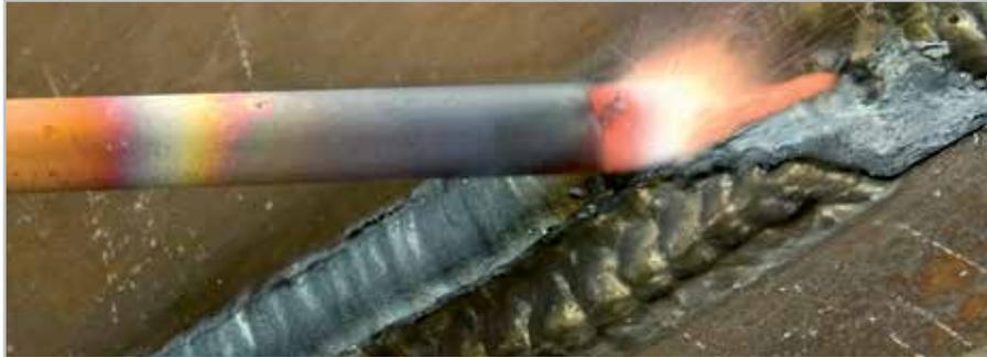
KempGouge ARC 800 makes easy work of carbon arc gouging tasks.
